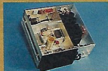
Chassis of the SB-230. Note massive built-in power supply, completely shielded final, cage, and safety interlock.
