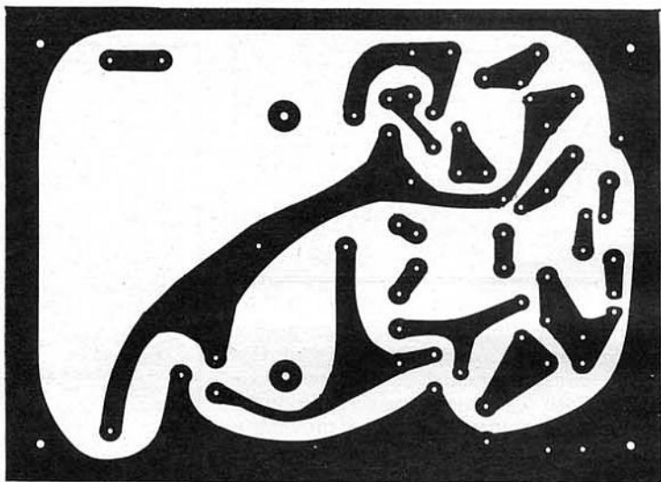
Fig. 5. Actual-size photo of amplifier printed circuit board can be copied or the board can be purchased etched and drilled (see note in Parts List).
