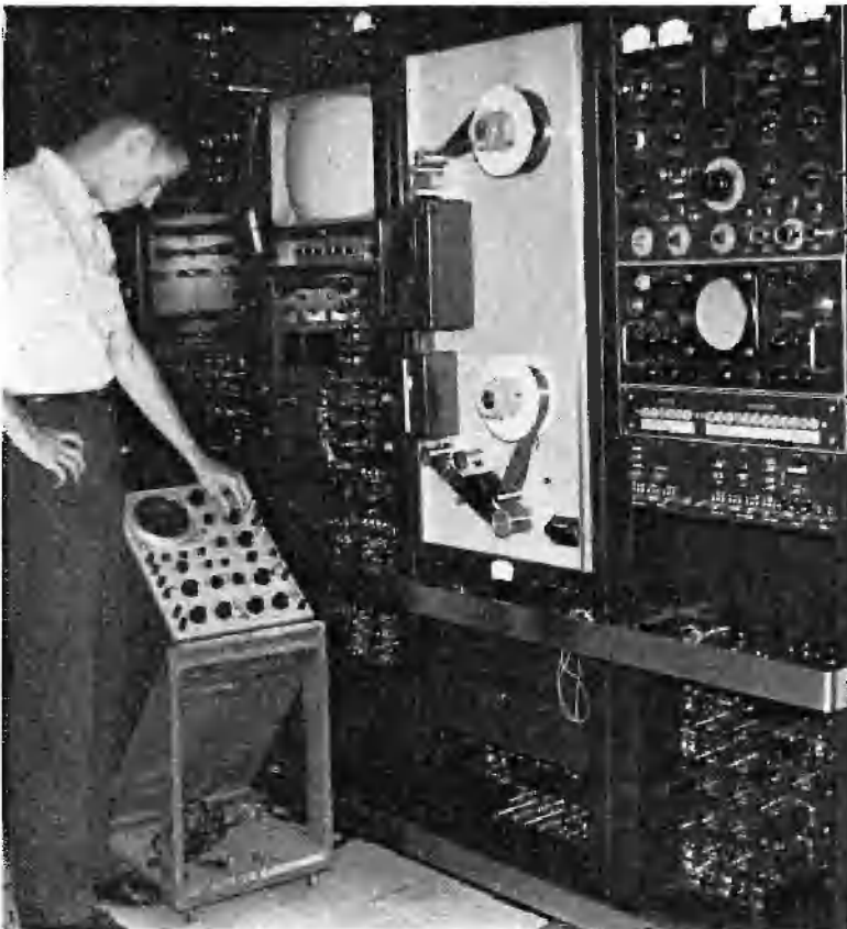
FIG. 11. RCA TRT-1B TV Tape facility in the control room at the downtown studios. WTVM uses this recorder for commercial spots and programs.
